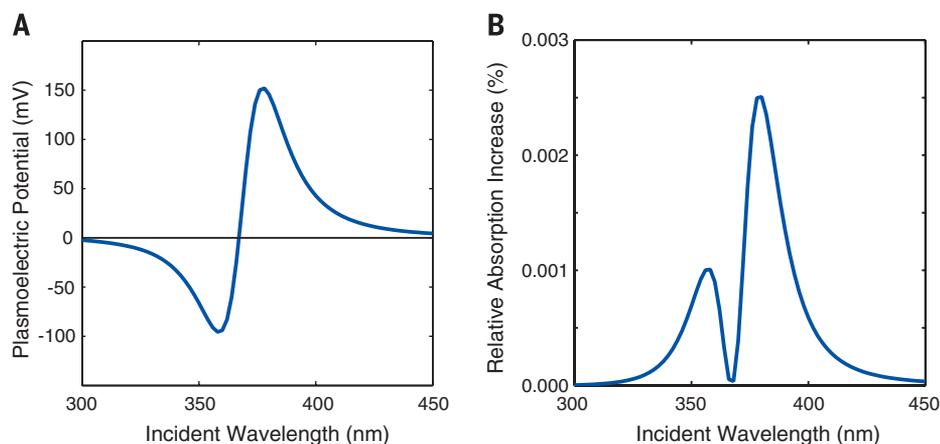
**Fig. 3. Modeled plasmoelectric response for Ag nanoparticles.** A 20-nm-diameter Ag particle in vacuum is illuminated with monochromatic light ( $1 \text{ mW/cm}^2$ ). (A) Plasmoelectric potential and (B) relative absorption increase as a function of incident wavelength.
