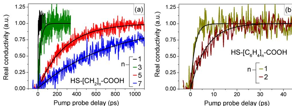
**Figure 3.** ET kinetics between  $\sim 3$  nm CdSe QDs and  $\text{SnO}_2$  through (a)  $n$ -methylene based bridges ( $\text{HS}-[\text{CH}_2]_n-\text{COOH}$ , with  $n = 1, 3, 5, 7$ ) and (b)  $n$ -phenylene based bridges ( $\text{HS}-[\text{C}_6\text{H}_4]_n-\text{COOH}$ , with  $n = 1, 2$ ). Black lines depict single exponential fits.
