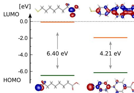
**Figure 5.** Energetic and spatial distribution of the frontier orbitals of  $\text{HS}-[\text{CH}_2]_7-\text{COOH}$  (left) and  $\text{HS}-[\text{C}_6\text{H}_4]_2-\text{COOH}$  (right) molecules, calculated using DFT (see the Supporting Information).
