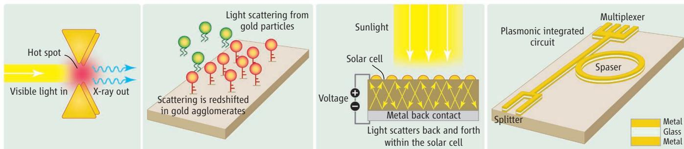
**Applied plasmonics.** (Left) A plasmonic hot spot between metal nanoparticles creates soft x-rays. (Middle left) Measuring the resonance shift in coupled metal nanoparticles leads to efficient sensing. (Middle right) Scattering from
