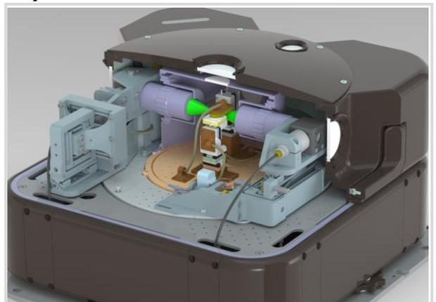
Figure 2. Our tunable cavity in a closed-cycle cryostat with free-space optics.
