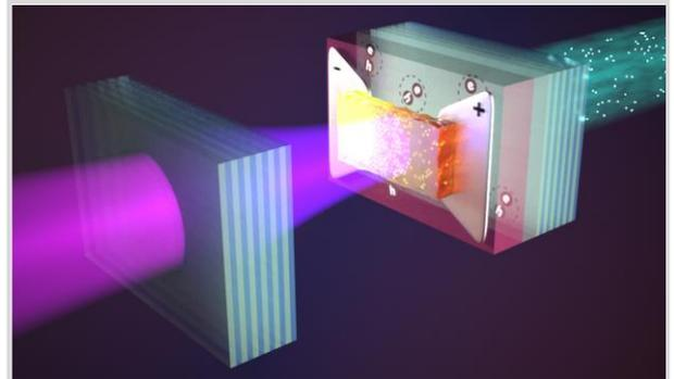
Figure 1. An optical cavity contains 2 semiconductors, one hosting excitons (under the electrodes) and another conducting charges. Light-induced superconductivity has been predicted for this system.
